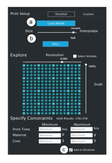
Figure 5: Adding a new model: (a) load model geometry (.stl), (b) SliceHub slices 10% of the print profile and model scale combinations and interpolates the rest, (c) SliceHub checks if users allowed sharing the model on the repository and then uploads the model and slicing results.
