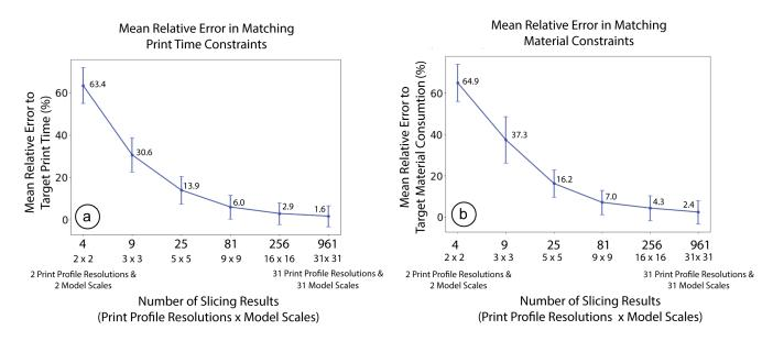
Figure 6: Mean relative error for different numbers of print resolution profiles and model scales offered in the user interface when either (a) a print time constraint or (b) a material amount constraint need to be matched.
