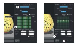
Figure 3: User Interface (Ultimaker Cura Plugin): (a) load .zip file (3D model (.stl) and meta-data (.json)), (b) UI updates to display print time and material consumption for each print profile resolution and model scale. (c) Adding lower and upper bounds for print time or material consumption shows only valid configurations. (d) Slicing the preferred configuration to generate the .gcode file for 3D printing.
