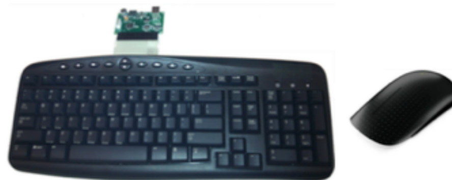
Figure 1. Pressure-sensitive keyboard (left), and capacitive mouse (right).
