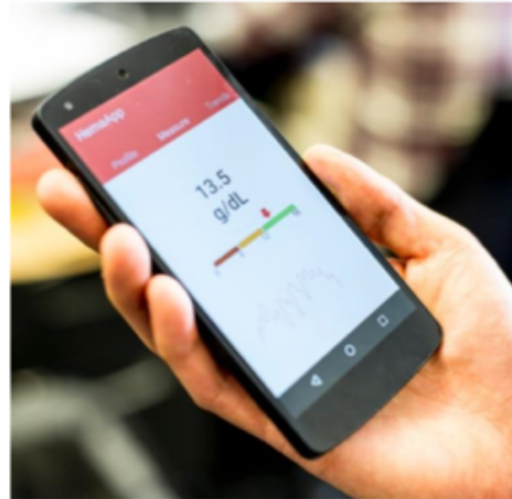
Figure 1. HemaApp is a smartphone application that measures the hemoglobin level using the phone's built-in camera and white flash LED.
