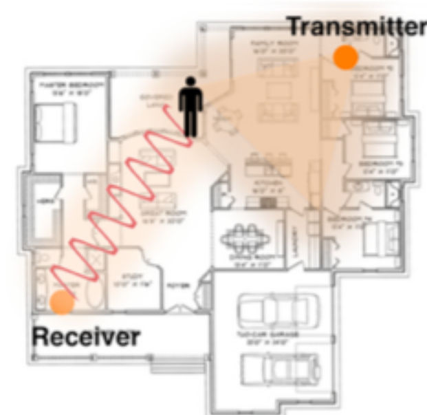
Figure 1: WiBreathe can detect a person's respiration rate from anywhere in a house without any instrumentation on the body. The system only requires a pair of transmitter and receivers that can be placed anywhere in the house.
