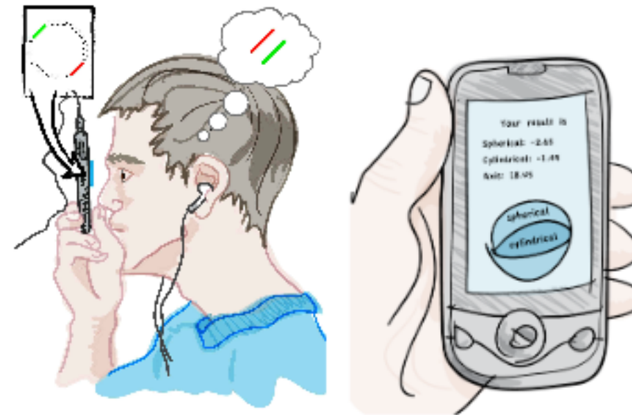
Figure 1: Can a person look at a portable display, click on a few buttons and recover his refractive fidelity? Our solution combines inexpensive optical elements, programmable display and interactive software components to create the equivalent of a parallax barrier display that interfaces with the human eye. Using this platform, we create a new range of interactivity for measuring several parameters of the human eye, such as refractive errors, focal range, and focusing speed.
