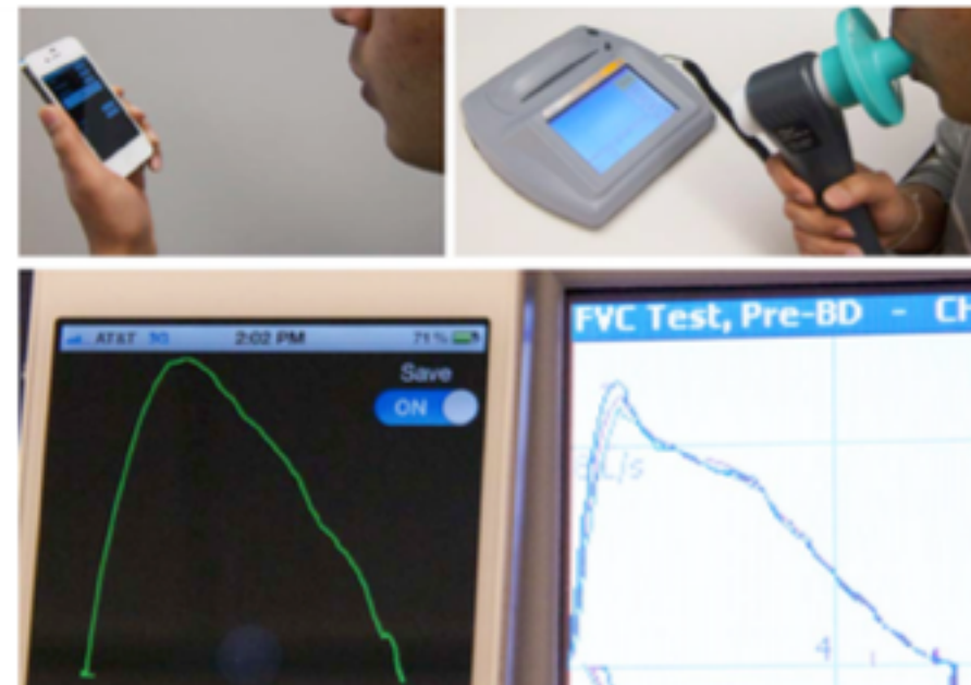
Figure 1. Subjects using SpiroSmart (left) and a clinical spirometer (right) and example curves from each device.
