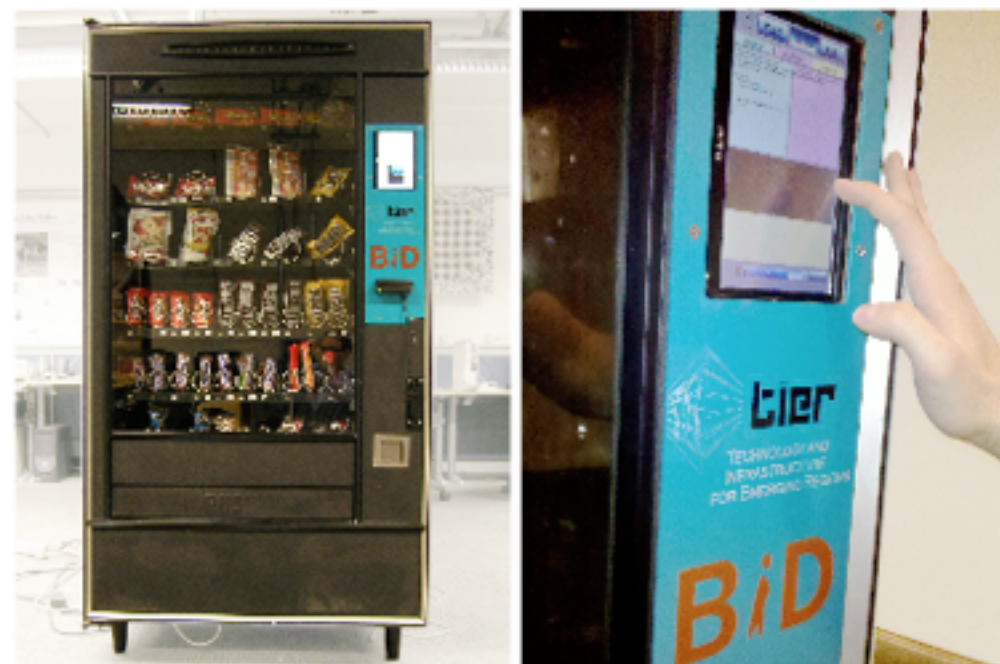
Figure 1. With Umati, the communitysourcing vending machine, users complete tasks on a touchscreen and receive non-monetary rewards.
