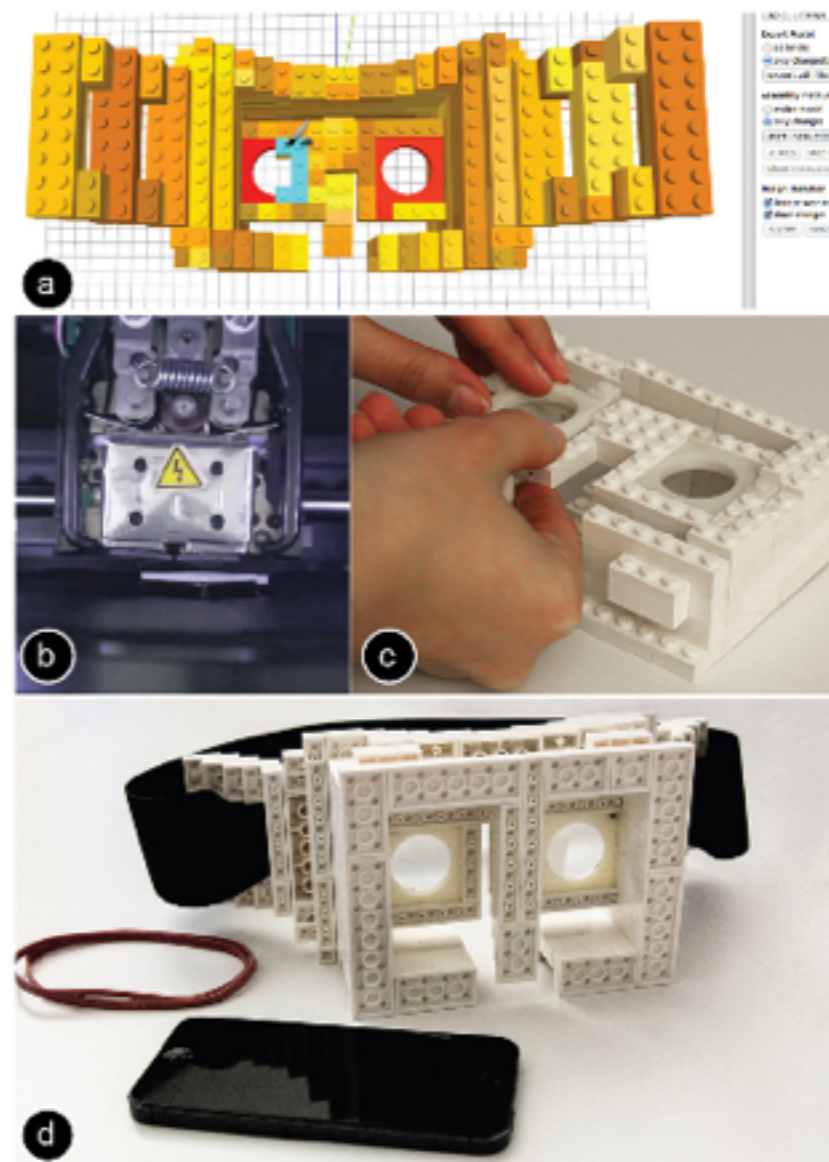
Figure 1: Let's fabricate this head-mounted display body quickly: (a) The exact shape of the lens mounts matters; the user thus marks them as “high-resolution” in faBrickator and (b) prints them. (c) faBrickator shows the user how to create everything else from Lego
