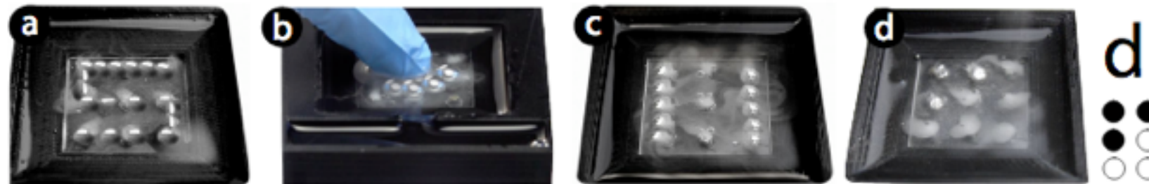
Figure 1. (a) A (timelapsed) visual display showing animated letter “S” using locomotion, and (b) a (timelapsed) tactile display with direction feedback using vibration and locomotion of a liquid metal drop. (c) A timelapsed visio-tactile equalizer widget and (d) a dynamic Braille display.
