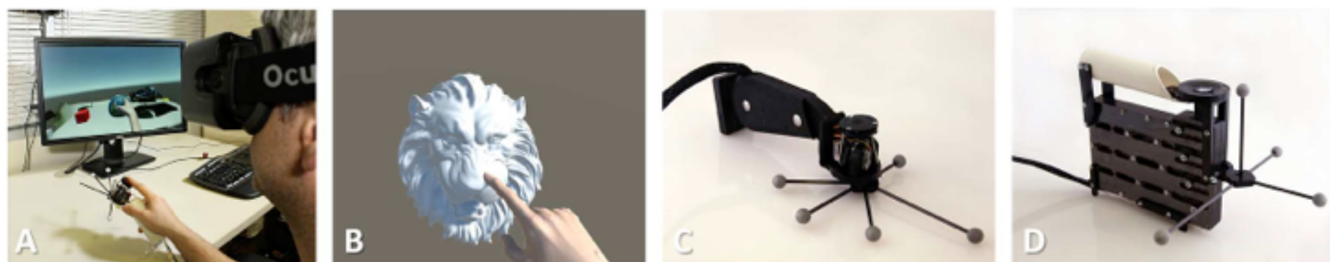
Figure 1: (a) Our 3D haptic shape controllers allow the Virtual Reality user to touch and feel what they would otherwise only see. (b) Our controllers enable users to explore virtual 3D objects with their finger. (c) NormalTouch renders the surface height and orientation using a tiltable and height-adjustable platform. (d) TextureTouch renders the detailed surface texture of virtual objects using a 4×4 pin array, which users experience on their finger pad.
