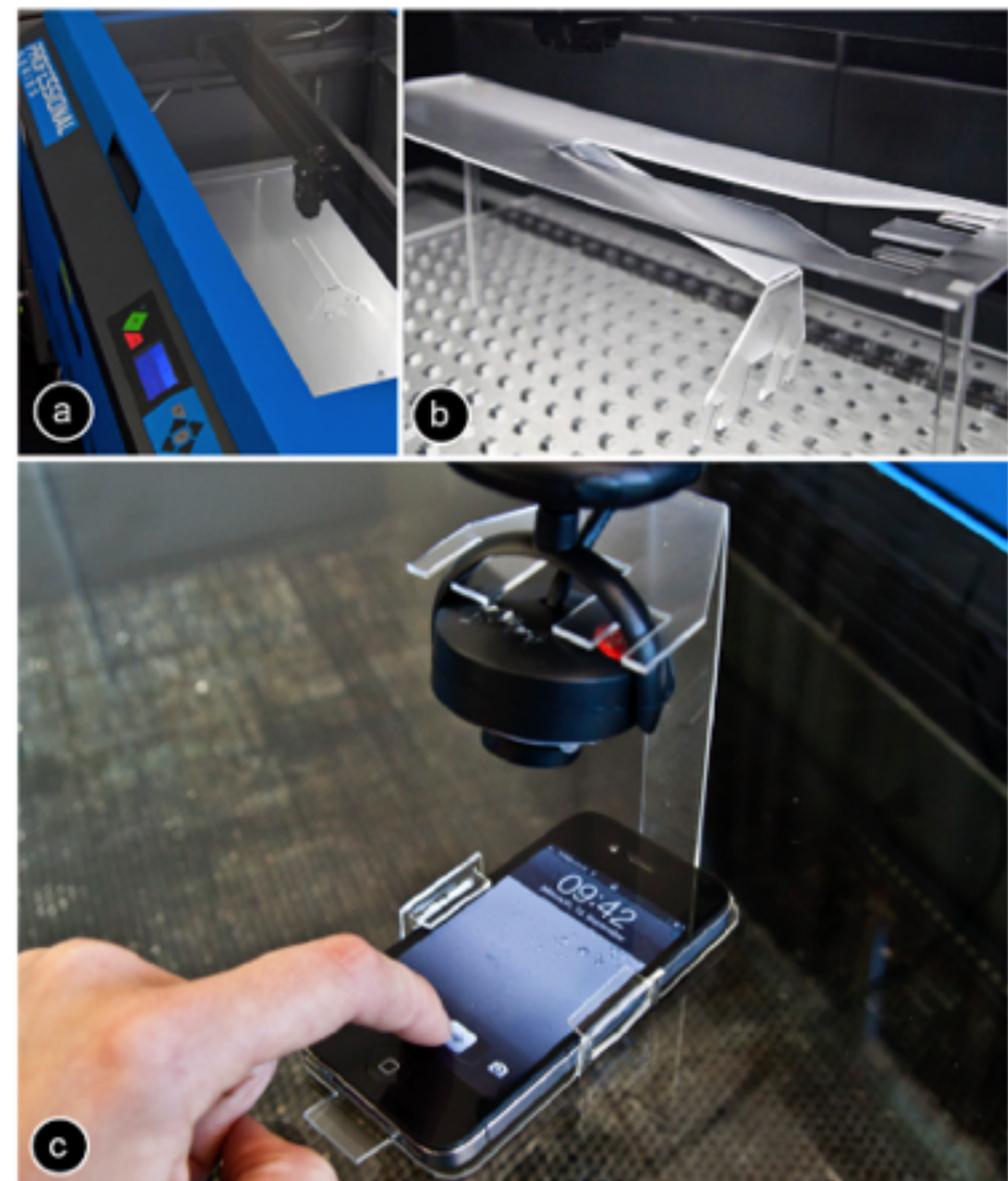
Figure 1: LaserOrigami fabricates 3D structure by bending, rather than using joints, thereby eliminating the need for manual assembly. Here it fabricates a mobile phone screen cam by (a) cutting the contour lines
