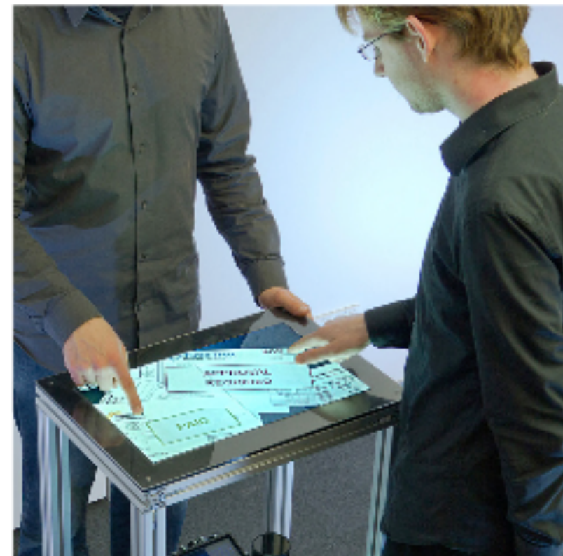
Figure 1: Fiberio is a rear-projected tabletop system that identifies users based on their fingerprints during each interaction —unobtrusively and securely. The shown application uses this to verify that the respective user has the authority to perform the current activity, here approve invoices above a certain value. The key that allows Fiberio to display an image and sense fingerprints at the same time is its screen material: a fiber optic plate.
