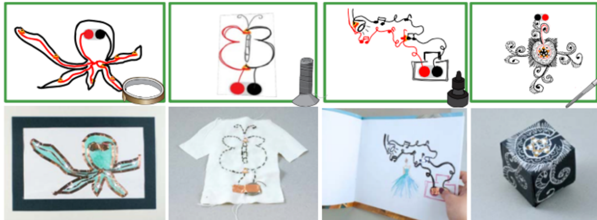
Figure 1. Sketched digital circuits (top), and fabricated circuits (bottom) created through various craft mediums: a) copper tape painting on paper, b) sewn conductive thread on fabric, c) painted graphite ink as interactive illustration, and d) decorative silver ink to ornament physical objects.
