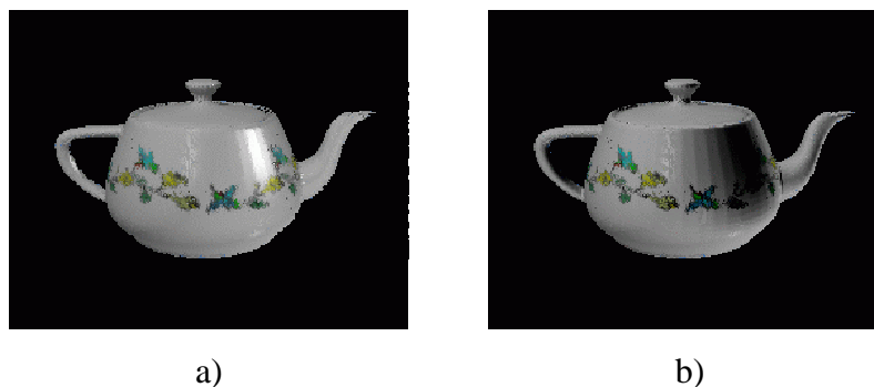
FIGURE 6.5 Phong shading. a) Adding a specular highlight to the upper-right of a teapot. b) Subtracting light from the same region.
