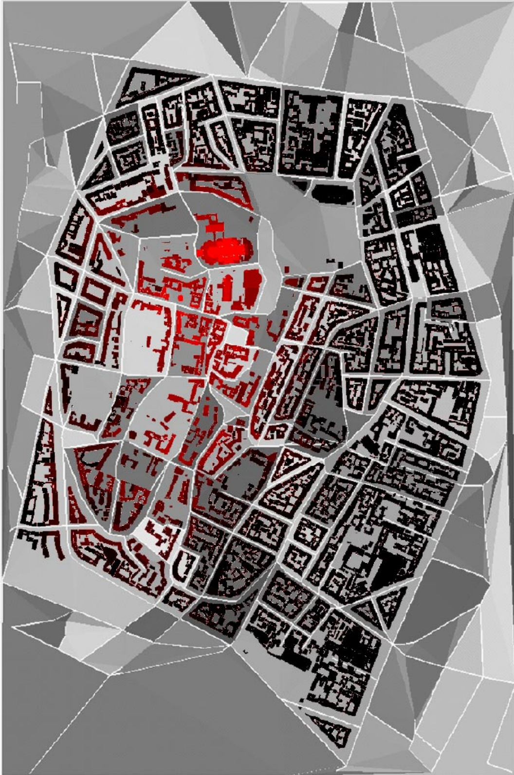
Figure 7-7: An overhead view of the Paris model: encoded in the buildings are their relative heights. Dark red buildings represent the lowest buildings while bright red buildings represent the tallest buildings.
