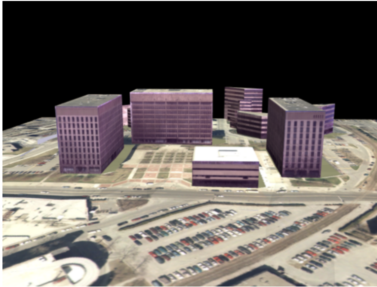
Figure A-5: The 3D CAD model of Tech Square generated by Coorg's Vertical Facade Extraction Algorithm and converted to Alias format for rendering.
