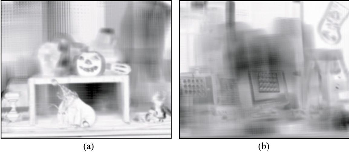
Figure 4-14: Visualizations of the \sigma scores used on the front (a) and back (b) focal planes for the picture in Figure 4-9. The closer to white, the better the score \sigma , which means objects are likely to be located near that plane.
