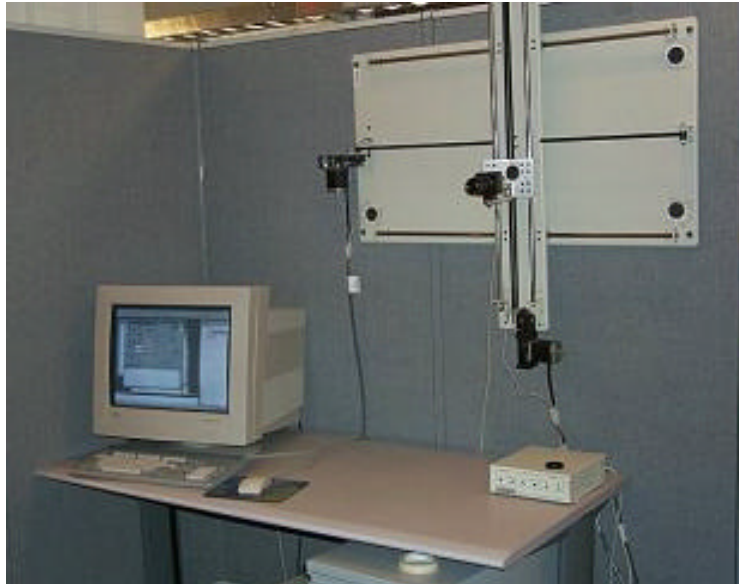
Figure 2: Camera Mounted on a Precision Robotic Gantry
