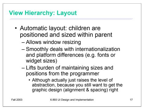
The view hierarchy is also used to direct the **layout** process, which determines the extents (positions and sizes) of the views in the hierarchy. Many GUI systems have supported automatic layout, including Motif (an important early toolkit for X Windows), Tk (a toolkit developed for the Tcl scripting language), and of course Java AWT.
