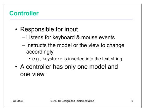
Finally, the controller handles all the input. It receives keyboard and mouse events, and instructs the model to change accordingly. For example, the controller of a text box receives keystrokes and inserts them into the text string.
