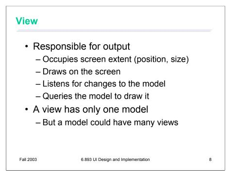
In MVC, view objects are responsible for output. A view occupies some chunk of the screen, usually a rectangular area. Basically, the view queries the model for data and draws the data on the screen. It listens for changes from the model so that it can update the screen to reflect those changes.
