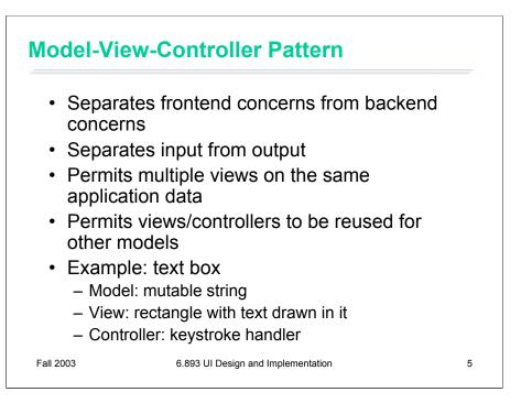
The **model-view-controller** pattern, originally articulated in the Smalltalk-80 user interface, has strongly influenced the design of UI software ever since. In fact, MVC may have single-handedly inspired the software design pattern movement; it figures strongly in the introductory chapter of the seminal "Gang of Four" book (Gamma, Helm, Johnson, Vlissides, *Design Patterns: Elements of Reusable Software*).
