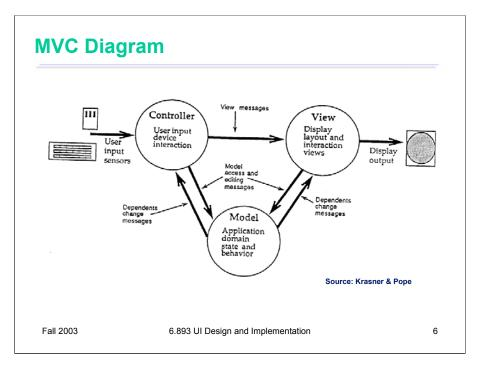
Here's a schematic diagram of the interactions between model, view, and controller. (Figure taken from Krasner & Pope, "A Description of the Model-View-Controller User Interface Paradigm in the Smalltalk-80 System", *JOOP* v1 n3, 1988).
