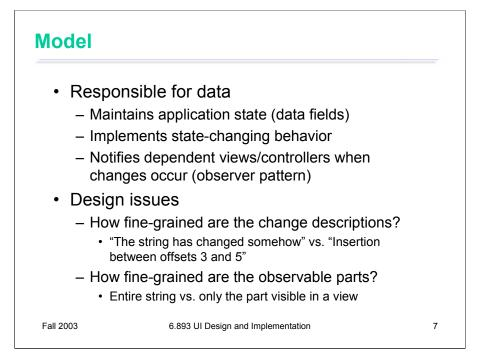
Let's look at each part in a little more detail. The model is responsible for maintaining applicationspecific data and providing access to that data. Models are often mutable, and they provide methods for changing the state safely, preserving its representation invariants.
