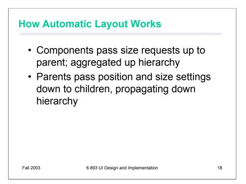
Whereas the view hierarchy was used in a top-down direction for drawing, and bottom-up for event propagation, automatic layout uses both directions. Here's how a typical automatic layout process works.
