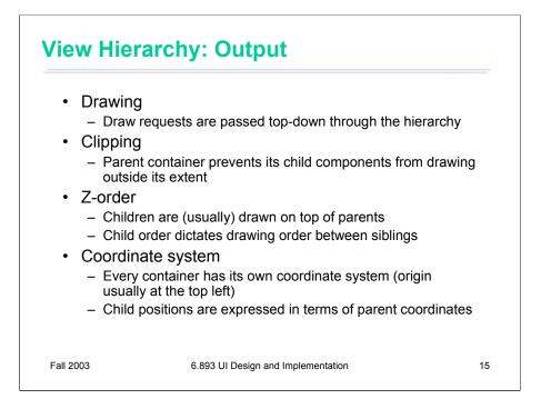
First, and probably primarily, the view hierarchy is used to organize output: drawing the views on the screen. **Draw requests** are passed down through the hierarchy. When a container is told to draw itself, it must make sure to pass the draw request down to its children as well.
