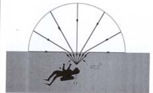
Fig. 3.7B The optical manhole. Light from the horizon (angle of incidence = 90°) is refracted downward at an angle of 48.6°. This compresses the sky into a circle with a diameter of 97.2° instead of its usual 180°.
