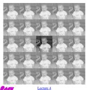
First, it assumes that the image tiles an infinite plane. This leads to a transform that contains both even (cosine-like) and odd (sine-ike) components.
