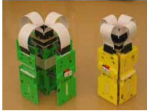
Fig. 2. Two modules of the Crystal robot: the one on the left is fully expanded and the one on the right fully contracted.
