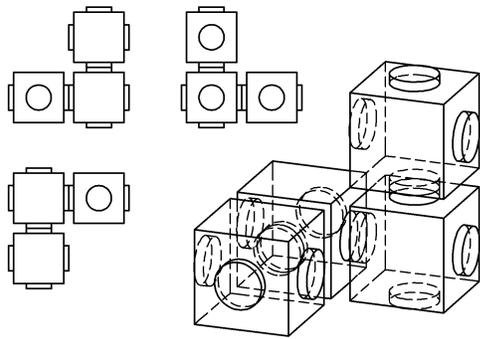
Fig. 6. By using distinct types of pebbles capable of bonding in either the X-Y, X-Z, or Y-Z planes we can create 3D structures using only four connectors per module.
