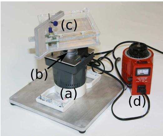
Fig. 3. To aid in self-assembling, we built a simple vibration table from a \$100 back massager (a) and a Panavise universal joint (b) which allows us to control the angle of the assembly table (c). A variac (d) allows us to control the speed of vibration.
