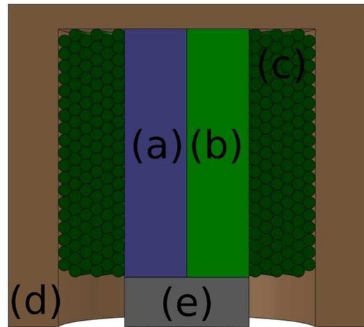
Fig. 5. An axially symmetric electropermanent magnet could be created by placing two half round magnets (a,b) next to each other to form a core that is then wound with a coil (c) and placed inside of a ferromagnetic cup (d). A small cap (e) is attached to the exposed end of the magnetic core to prevent fringing fields from giving rise to attractive forces when the EP magnet is deactivated.
