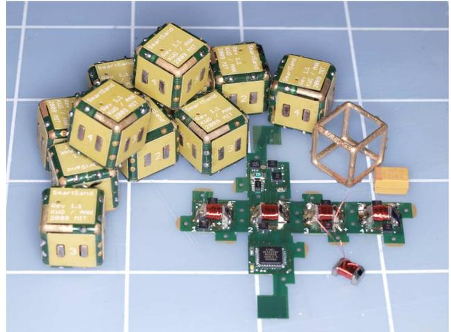
Fig. 1. Each programmable matter pebble is a 12mm per side, and together they are able to form complex 2D shapes using four electropermanent magnets able to hold 85 times the individual module weight. The pebbles are formed by wrapping a flexible circuit around a brass frame. An energy storage capacitor hangs between two tabs occupies the center of the module.
