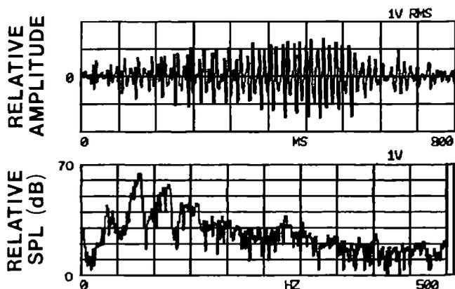
FIG. 3. Waveform (upper) and spectrum (/Hz, lower) of a complex moan having a weak 35-Hz fundamental and pulsive AM. Analysis bandwidth, 1.9 Hz.
