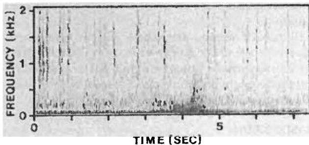
FIG. 6. Sonogram of broadband pulse train. Analysis bandwidth, 19 Hz.
