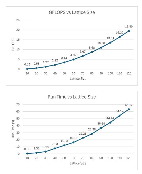
Figure 6.7: Graphs showing how the GFLOPS and runtime change as the lattice size (N) increases for the Dibaryon Hexaquark case study.
