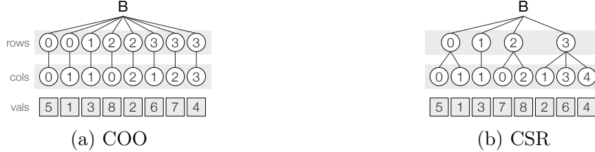
Figure 2-2: Coordinate hierarchy representations of the same sparse tensor stored in two different formats.
