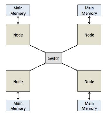
Figure 2-9: Switch-based distributed system.
