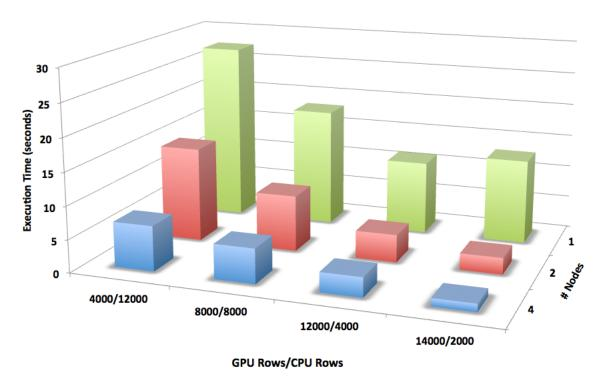
Figure 5-3: 3D chart for blur with cooperative execution using asynchronous execution and communication.
