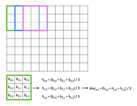
Figure 1-1: 2D blur example showing three consecutive applications of the stencil, as well as the computation for the blur of the upper left pixel.
