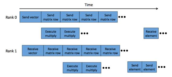
Figure 2-14: Timeline showing overlapping communication and computation with non-blocking functions.
