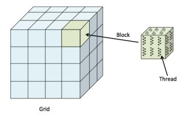
Figure 2-17: Grid, block, thread hierarchy.
