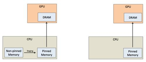
(a) Copying to GPU DRAM with a staging (b) Copying to GPU DRAM without having copy required first.
