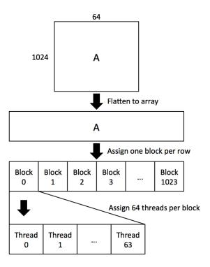
Figure 4-7: Mapping matrix  $\tt A$  as a 1D grid of 1024 1D blocks, each containing 64 threads. Matrices  $\tt B$  and  $\tt C$  would be similarly mapped.
