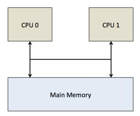
Figure 2-3: UMA (uniform memory access) configuration.
