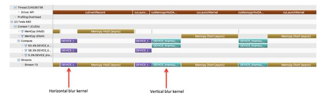
Figure 5-1: Timeline for synchronous execution of the blur.
