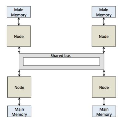
Figure 2-8: Bus-based distributed system.
