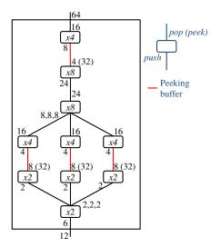
**Figure 1.** A stream graph, annotated with each worker's data rates. The *xN* in each worker denotes the number of executions of that worker in one possible schedule. In this schedule, the graph has overall pop rate 64 and push rate 12, i.e., it consumes 64 items and produces 12 items per execution of the schedule.
