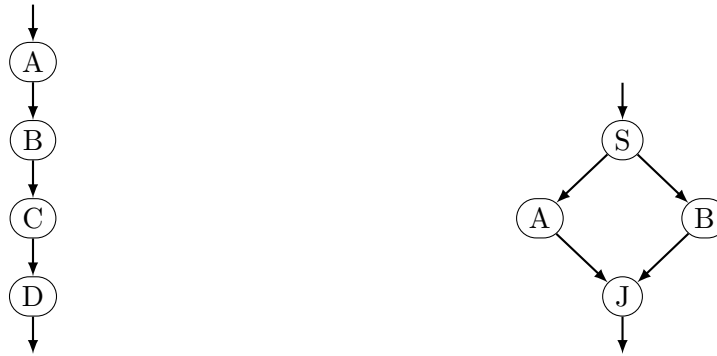
(a) Pipelines compose one-to-one elements (filters, pipelines or splitjoins) by connecting each element's output to the input of the next element. (b) Splitjoins compose a splitter, a joiner, and one or more one-to-one elements (filters, pipelines or splitjoins) by connecting the splitter's outputs to the inputs of the branches and the outputs of the branches to the joiner's input.
