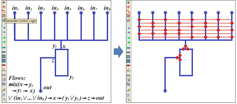
**2. Routing.** After the designer has indicated the positions of external control ports on the chip, Micado automatically connects each control line to a control port while respecting the design rules. The total length of the routes is minimized. Also, the number of corners (changes of direction) of control lines is reduced to yield an aesthetic outcome for the designer.
