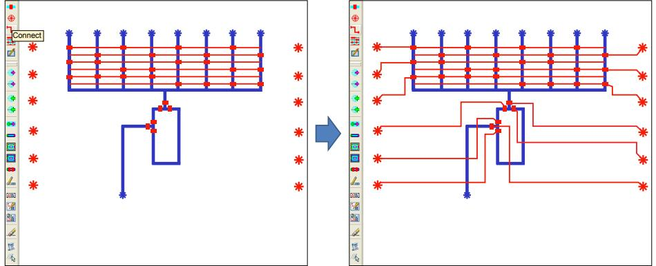
**3. GUI Generation.** Micado exports a graphical user interface for operating a chip in the laboratory. In AutoCAD, the user draws buttons (shown in green) and graphically associates them with flows of interest. When a button is clicked at runtime, valves are toggled to enable the associated flow. At right, the clicked button routes fluids from the last input, through the bottom of the mixer, to the output. Open valves are shown in blue, while closed valves are shown in red.
