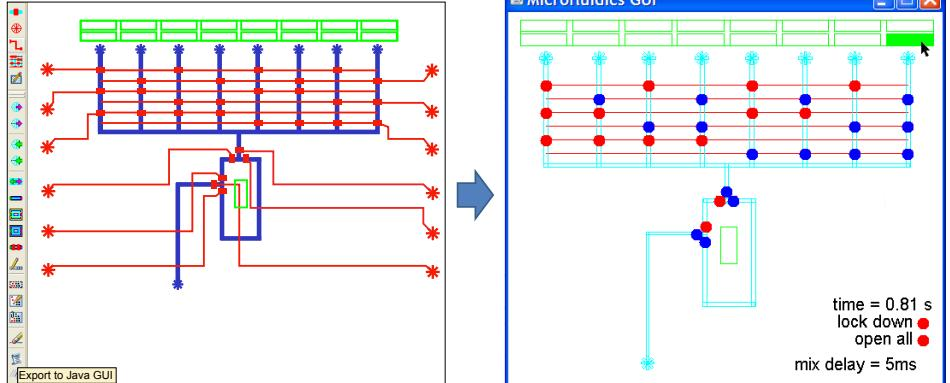
Fig. 2. Micado automates three key steps in the microfluidic design process: control inference, routing, and GUI generation.
