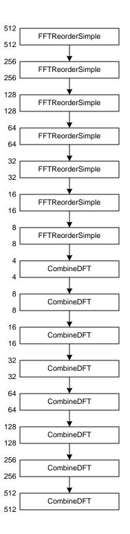
Figure 4-1: Stream graph for 256-element FFT. A single execution of the stream graph pops and pushes 512 floats, since each element is a complex number whose components are interleaved on tapes.
