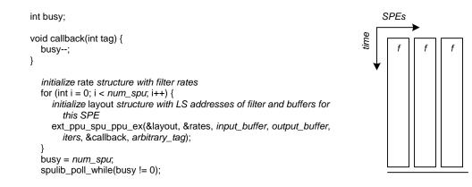
Figure 4-2: Pseudocode for running a data-parallel filter. The figure on the right represents the state of each SPE as time passes. The horizontal line indicates synchronization by the PPE.
