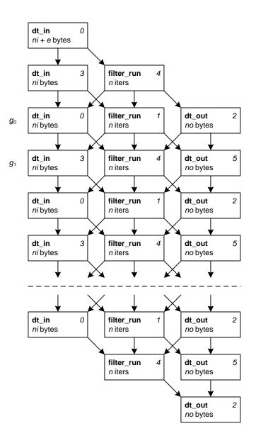
Figure 3-3: Sequence of commands to run a filter for a large number of iterations. Command IDs are indicated in the upper right. Each row is issued as a different group.
