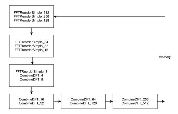
Figure 4-4: Pipelining FFT over six SPEs.
