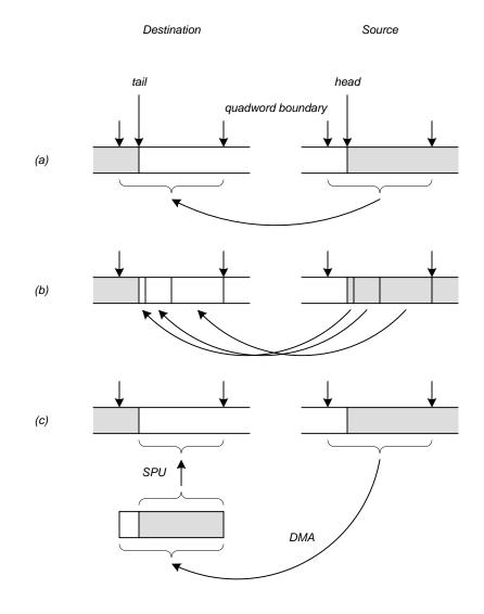
Figure 3-6: Different ways of handling unaligned data transfers. (a) is incorrect, since it overwrites data in the destination buffer with invalid data from the source buffer. (b) is correct but involves many DMA operations, and is less efficient. (c) is the actual method implemented.
