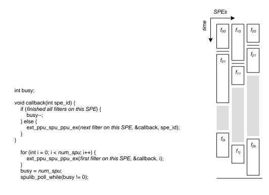
Figure 4-3: Pseudocode for running a course-grained software pipeline. The figure on the right represents the state of each SPE as time passes. Horizontal lines indicate synchronization by the PPE.
