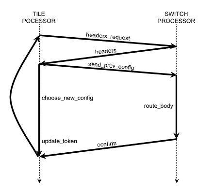
Figure 6-2: Phases of the Rotating Crossbar algorithm.
