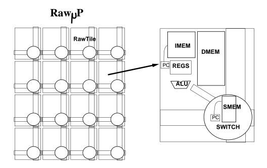
Figure 3-1: The Raw Processor with 16 tile processors in a  $4 \times 4$  grid.
