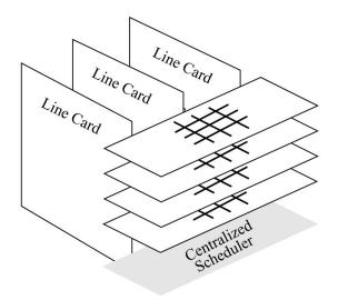
Figure 2-3: A four-way parallel crossbar switch, interconnecting multiple line cards. A centralized scheduler connects to each line card, and determines the configuration of the crossbar switch for each time slot (Adapted from [12]).
