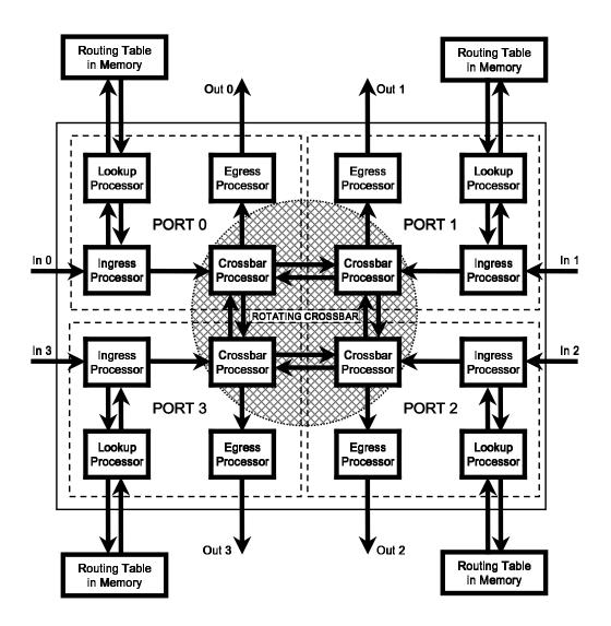
Figure 4-1: Mapping router functional elements to Raw tiles. Each of the four ports is comprised of four elements: an Ingress Processor, a Lookup Processor, a Crossbar Processor, and an Egress Processor.
