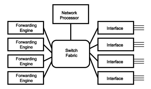
Figure 2-1: A typical router design.
