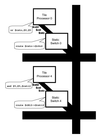
Figure 3-2: The switch and tile code required for a tile-to-tile send to the South from tile 0 to tile 4.
