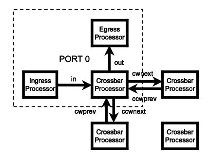
Figure 6-1: Network connections of a crossbar tile. Each Crossbar Processor has three incoming ("client") and three outgoing ("server") connections.
