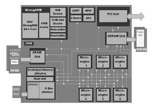
Figure 2-4: Intel IXP1200 network processor (Adapted from [1]).
