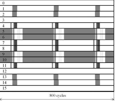
Figure 7-3: Utilization of the Raw processor on a per-tile basis. The top graph is for 64-byte packets, and the bottom graph is for 1,024-byte packets, both plotted for 800 clock cycles. The numbered horizontal lines correspond to Raw tile processors. Gray color means that a tile processor is blocked on transmit, receive, or cache miss.
