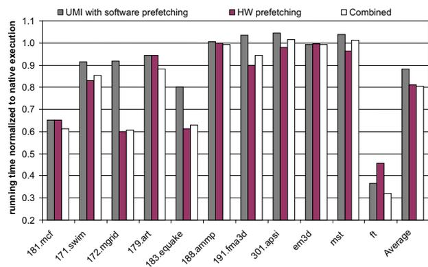
Figure 5. Running time on Pentium 4 with hardware prefetching enabled.
