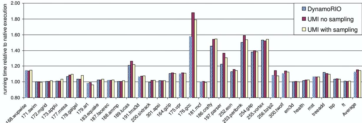
Figure 2. Runtime overhead on Pentium 4 with hardware prefetching enabled.
