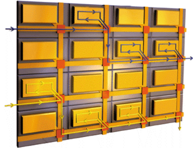
Diagram of a 4x4 Raw processor
