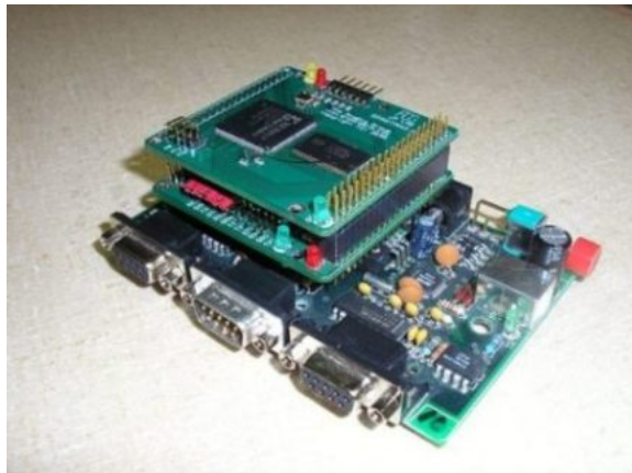
Fig. 2. The Microcontroller and FPGA boards are easily stacked on the CommPS board. The CommPS board provides both RS-232 and USB ports for communication with the Client PC.
