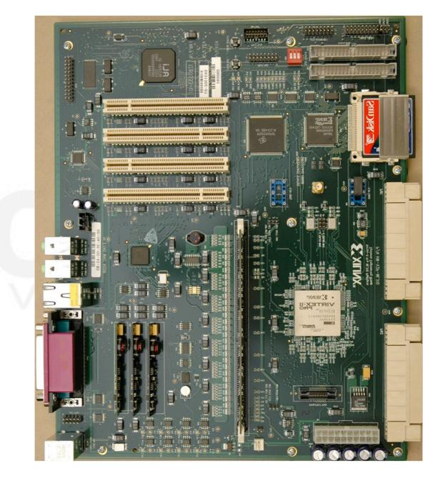
XC2VP30 FPGA with 2PowerPC 405 RISC Cores
