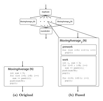
Figure 10: Fission of a filter that peeks.
