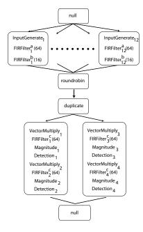
Figure 7: Stream graph of the load-balanced 12x4 Radar application. Vertical fusion is applied to collapse each pipeline into a single filter, and horizontal fusion is used to transform the 4-way splitjoin into a 2-way splitjoin. Figure 5 shows the benefit of these transformations.
