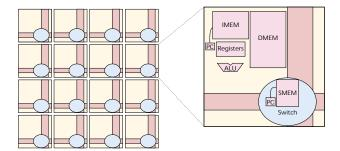
Figure 4: Block diagram of the Raw architecture.
