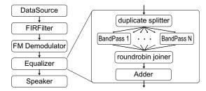
Figure 2: Block diagram of the FM Radio.
