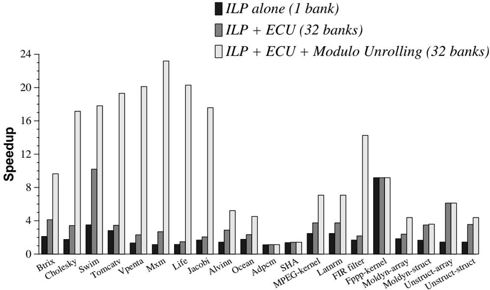
Figure 7: Comparison of 32-tile speedups using instruction-level parallelism (ILP) alone, ILP with ECU, and ILP with both ECU and modulo unrolling.
