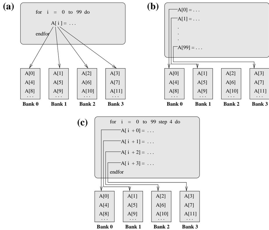
Figure 6: Example of modulo unrolling. (a) Original code. Array  $A$  is low-order interleaved on a 4-bank bank-exposed machine. The  $A[i]$  reference instruction goes to different banks for different values of  $i$ . (b) Code after full unrolling. Disambiguation is attained, but code size is huge. (c) Code after unrolling by factor 4. Disambiguation is attained with limited code size increase.
