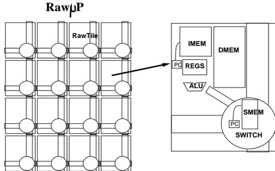
Figure 3: A Raw microprocessor is a mesh of tiles, each with a processing element, some memory and a switch. The processing element contains both registers and an ALU. The processing element interfaces with its local instruction memory, local data memory and local switch. The switch contains its own instruction memory.
