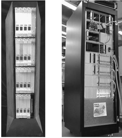
Figure 2: 16-node machine and 128-node chassis populated with a 32-node machine.
