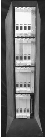
Figure 2: 16-node machine and 128-node chassis populated with a 32-node machine.
