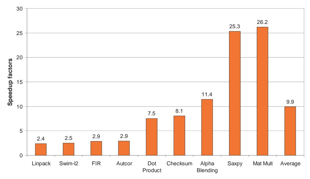
single SPE, optimized, automatic simdization vs. scalar code
