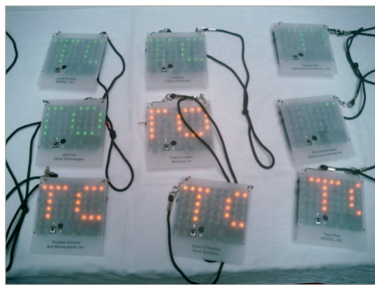
Figure 1: The Laibowitz and Paradiso Uberbadge. This badge-like platform allows social context sensing by IR, audio, and motion so that wearers can automatically bookmark interesting people and demonstrations, and it displays messages designed to build social networks.
