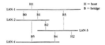
Let us first compute the cost of the ST approach. After *N* Hello message exchanges, where *N* is on the order of the network diameter [4], the topology will be pruned to the following spanning tree:
