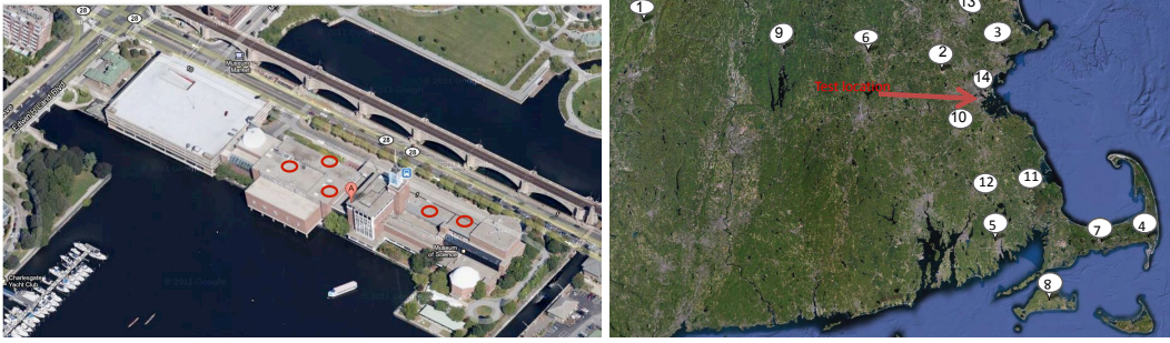
Figure 1: Left: Red circles show location of anemometers on rooftop of Museum of Science, Boston. Right: Neighboring-site data from fourteen airports (marked with circles) is used in the MCP correlation step.
